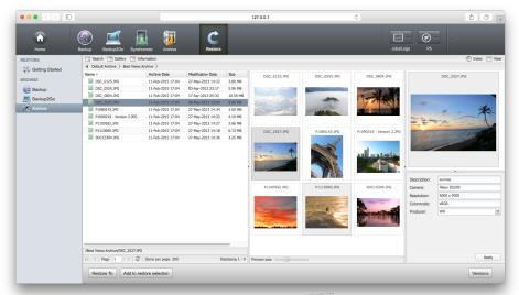
For day-to-day protection of production data, use part of the Qualstar library for regular, full or incremental backup with **Archiware P5 Backup**. Since the position of the files is stored the restore is as quick as possible. Parallelization of multiple drives provides maximum throughput.
