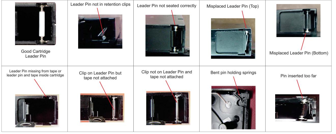
If the cartridge passes the visual inspection above, re-tension it using your software.
