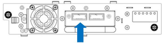
If you are using a SAS fanout cable, attach one mini-SAS connector into the connector on each tape drive. Any unused ends of the SAS fanout cable should be secured to the rack to minimize stress on the connectors and cable.
