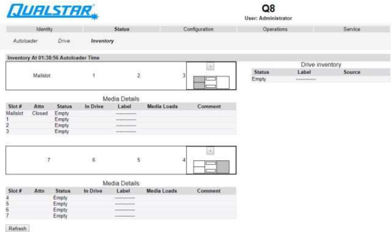
Figure 39 Tape cartridge inventory (detail)
