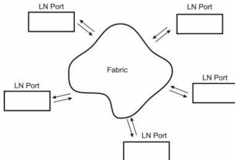
**Figure 7 Fibre Channel topology (LN Port)**
