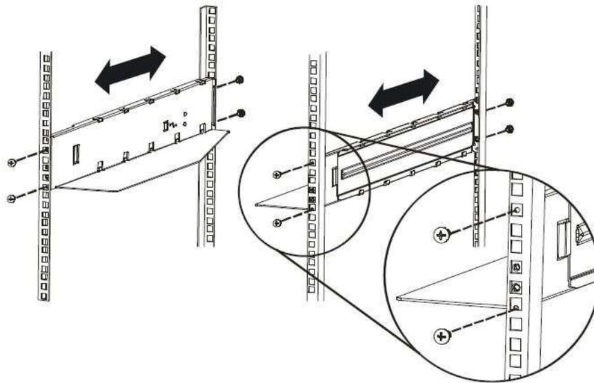
Figure 13 Install the rack rails
