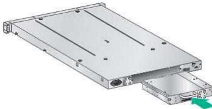
**Figure 17 Install a tape drive**
