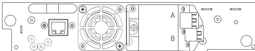
1. Remove the FC port caps if necessary. Attach one end of the FC cable to [Port A] on the tape drive.
