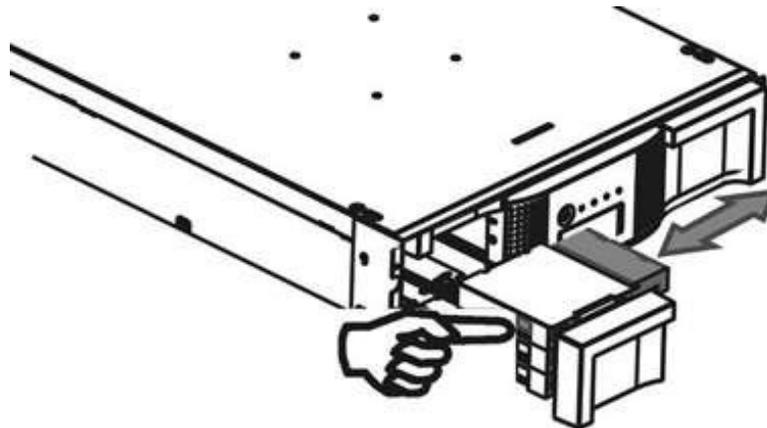
Figure 59 Removing a stuck tape
