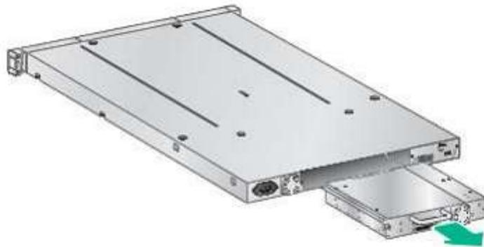
**Figure 64 Remove a tape drive**
