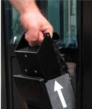
**Figure 6-13** Removing the I/O port magazine
