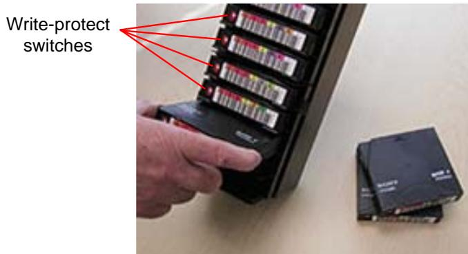
**Figure 6-9** Inserting cartridges into the I/O port magazine
