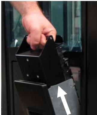
**Figure 6-8** Removing the I/O port magazine
