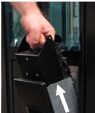
**Figure 6-4** Removing the I/O port magazine
