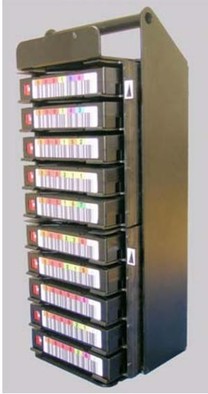
**Figure 2-15** I/O port magazine
