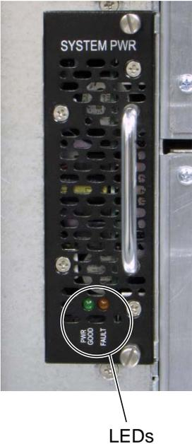
**Figure 15-3** Power supply LEDs
