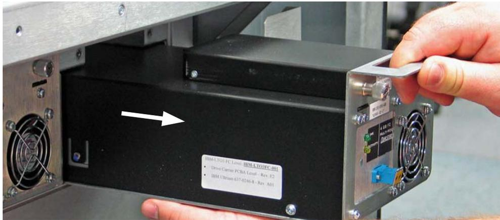
**Figure B-5** Removing a drive carrier from a drive bay
