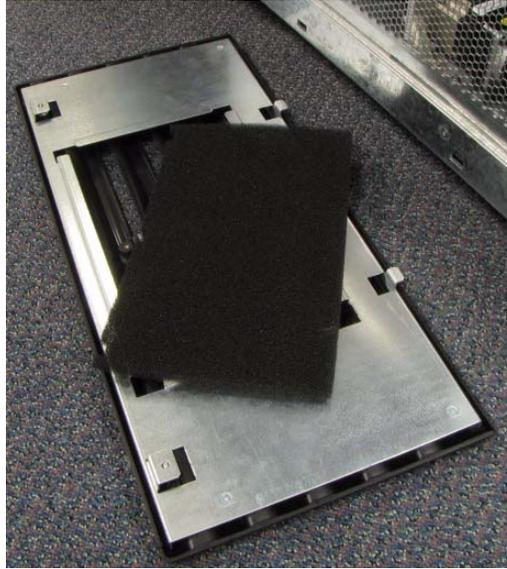
**Figure 16-6** Removing the air filter
