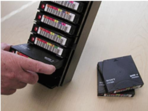
**Figure 6-14** Removing cartridges from the I/O port magazine
