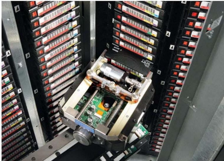
**Figure 2-9** Robotic handler (shown reaching into an attached MEM)
