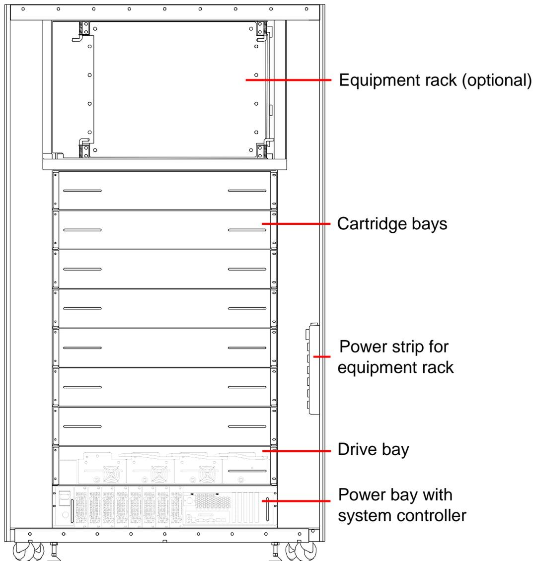
**Figure 2-3** Rear view of the LRM
