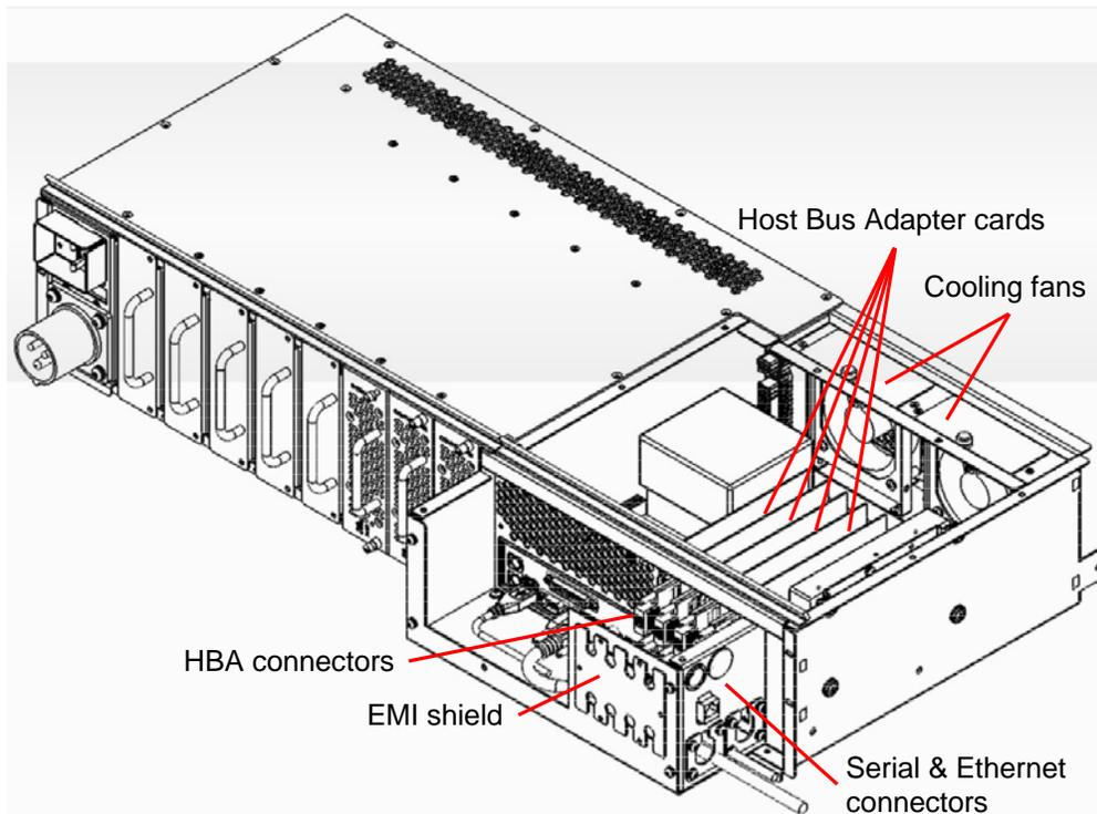
**Figure 2-4** Controller/power bay showing system controller components
