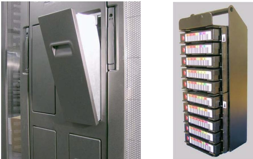
**Figure A-1** (left) One of up to four physical I/O ports (right) Removable 10-slot magazine
