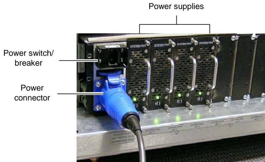
**Figure 2-5** Power supplies and power connector
