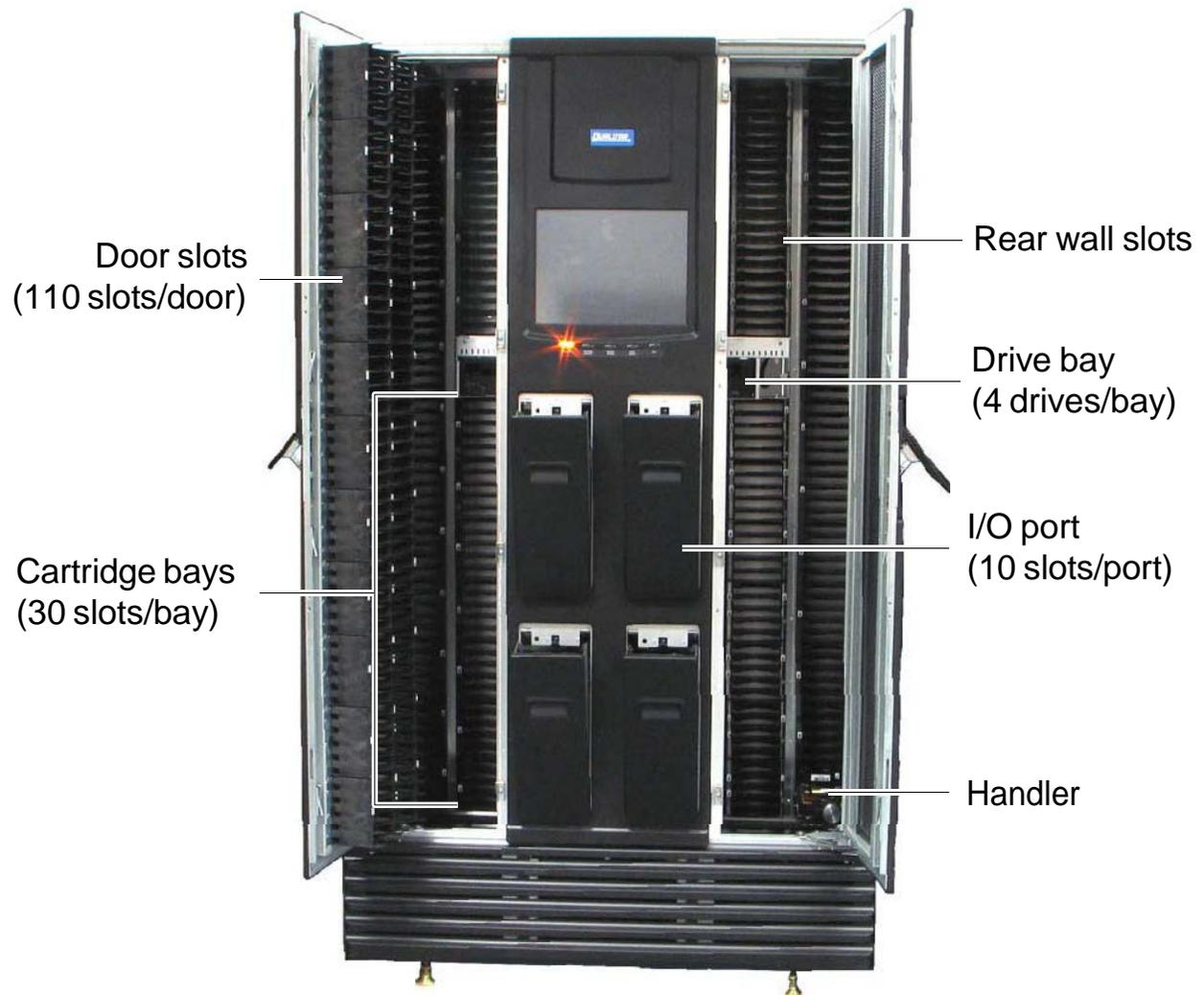
**Figure 2-2** Inside view of LRM (I/O ports shown open)
