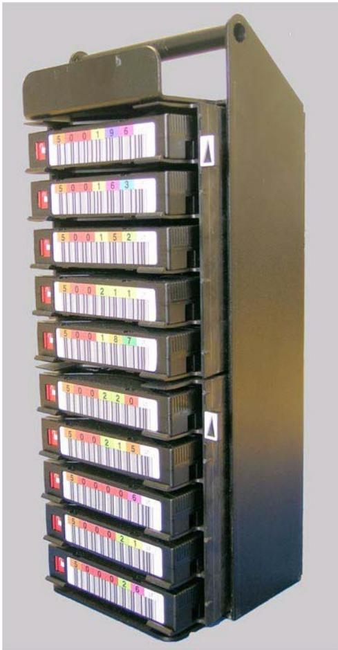
**Figure 2-11** I/O port magazine
