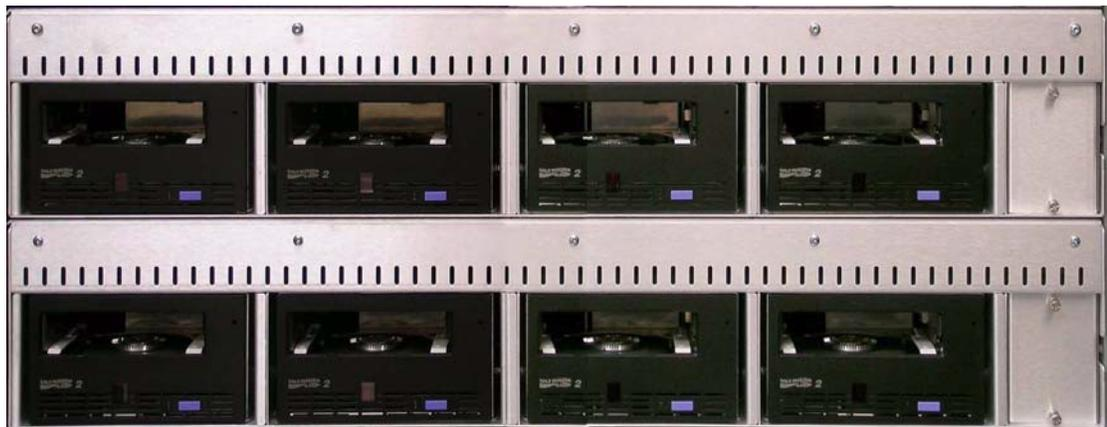
**Figure 2-8** Two drive bays (front panel removed)
