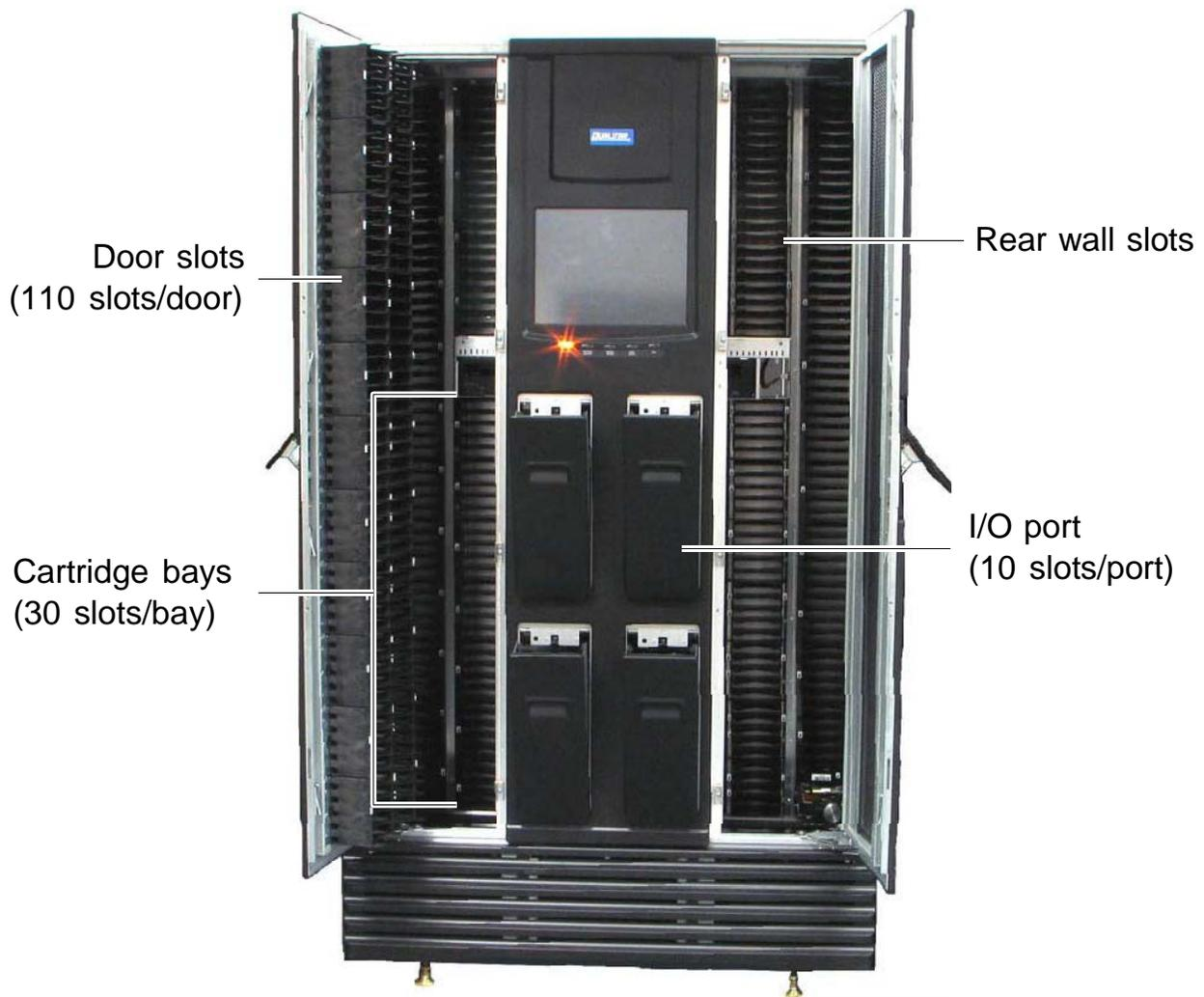
**Figure 2-12** Cartridge slots in LRM (front panel slots not shown)
