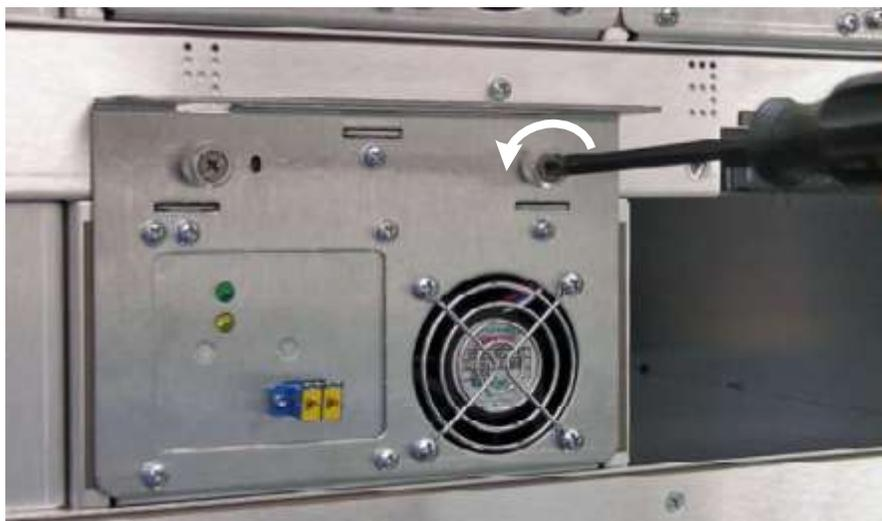
**Figure B-4** Loosening the tape drive assembly screws
