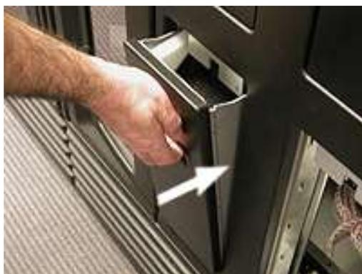
**Figure 6-12** Closing the I/O port
