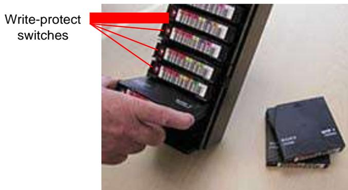
**Figure 6-5** Inserting cartridges into the I/O port magazine
