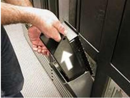
**Figure 6-4** Removing the I/O port magazine
