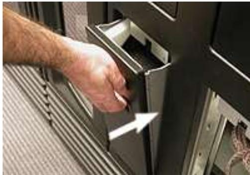
**Figure 6-7** Closing the I/O port
