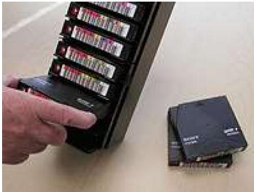
**Figure 6-10** Removing cartridges from the I/O port magazine
