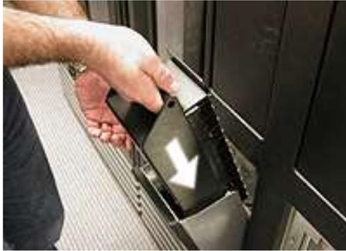
**Figure 6-6** Inserting the magazine into an I/O port
