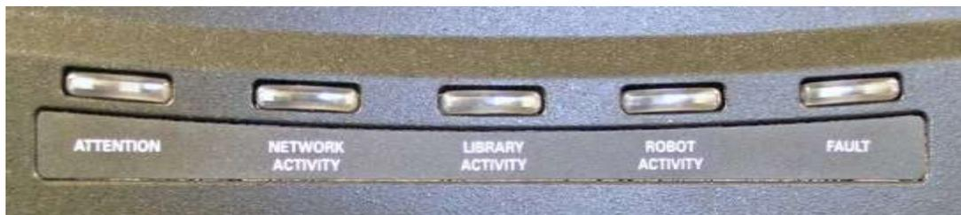
**Figure 15-1** Status LEDs on the LRM front panel
