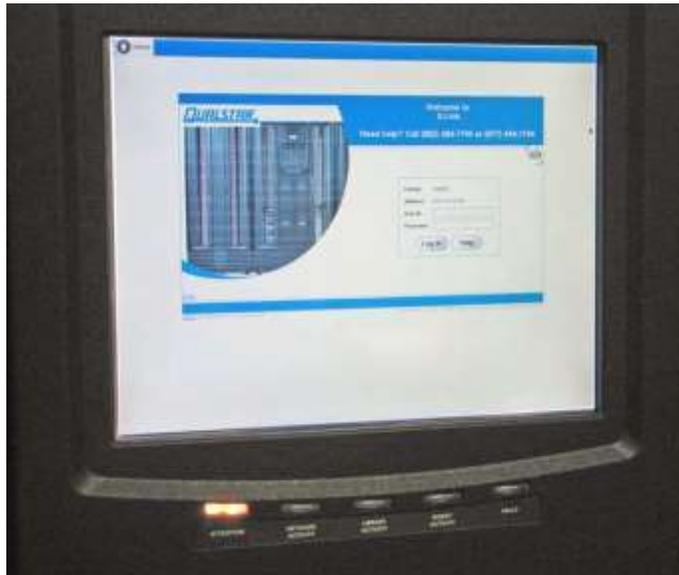
**Figure 2-10** Touch screen and status LEDs (X-Link log-in screen displayed)
