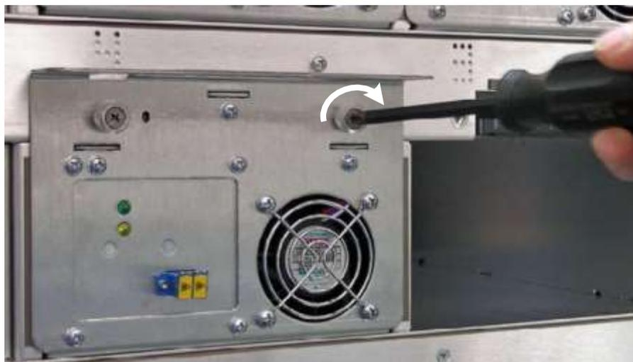
**Figure B-7** Tightening the tape drive assembly screws
