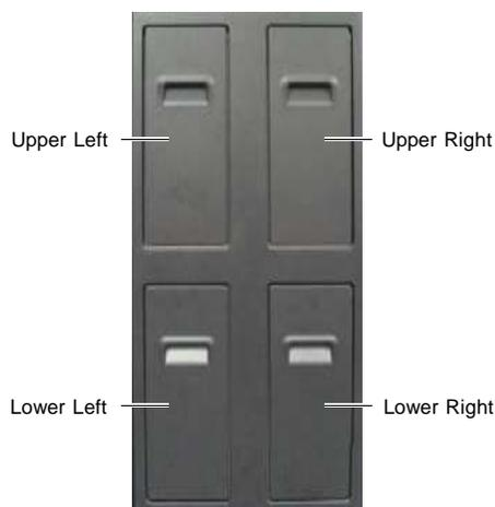
**Figure 11-6** Locations of the I/O ports
