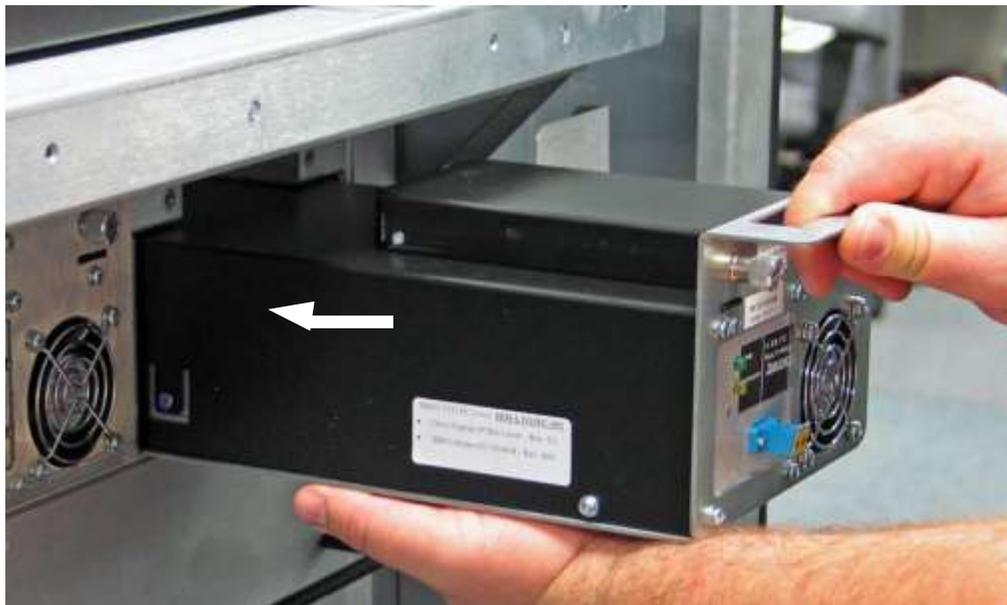
**Figure B-6** Inserting a tape drive assembly into a drive bay
