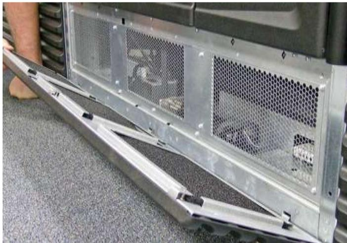
**Figure 16-5** Releasing the top edge of the grille (XLS-832700 shown)
