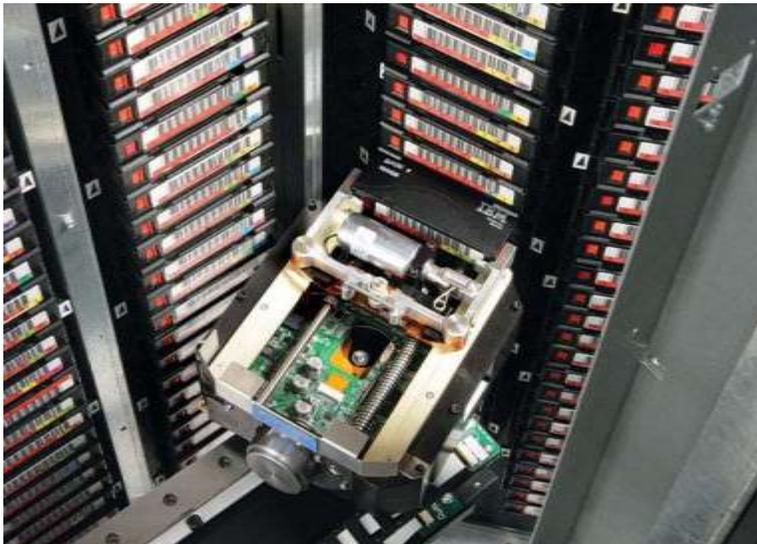
**Figure 2-12** Robotic handler (shown reaching into an attached MEM)
