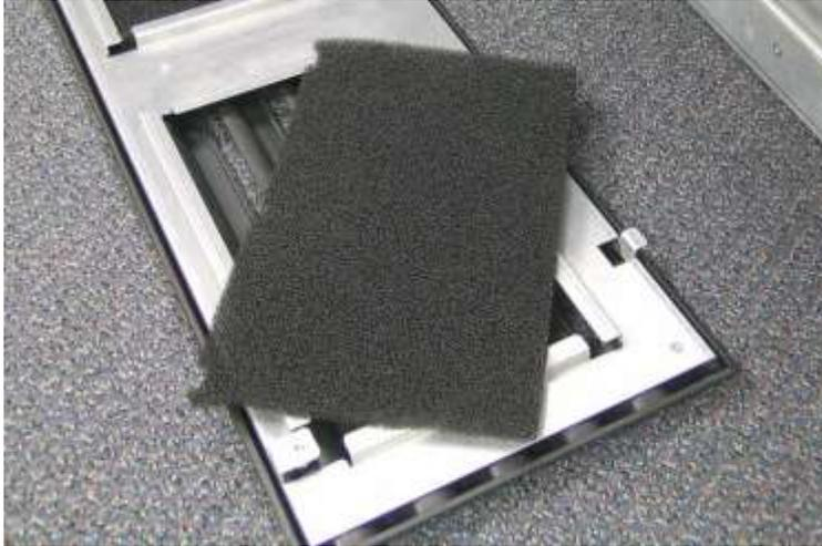
**Figure 16-6** Removing the air filter
