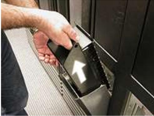
**Figure 6-9** Removing the I/O port magazine
