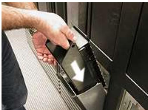
**Figure 6-11** Inserting the magazine into an I/O port
